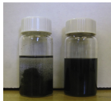
Fig. 12. Comparison of stability of nanocomposite suspension via ASP (left) and mASP (right). Material is PMMA-pCNT-1%.
